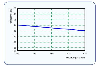
Reflection >93% avg from 450nm to 650nm, 15° thru 45° Reflection >93% in the P-plane of polarization @ 780 to 820nm, 10° thru 45°
