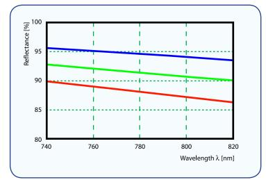
MAL400 measured at 45°. Red is P polarization, Blue is S polarization, and Green is average polarization
