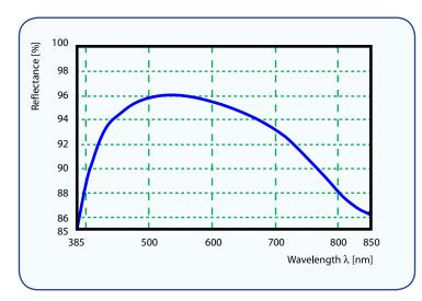
MAL200 measured at normal Angle of Incidenece.
