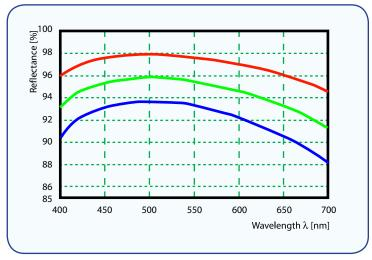
MAL200 measured at 45°. Red is S polarization, Blue is P polarization, and Green is average polarization.
