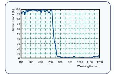
The average transmission is  $\geq$  93% from 425 to 675nm, and the average transmision is  $\leq$  5% from 750 to 1150nm at normal incidence.
