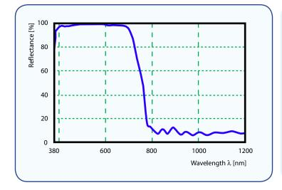
The average reflection is greater than 95% from 425 to 650nm, and the average reflection is less than 15% from 800 to 1200nm at 45° angle of incidence.
